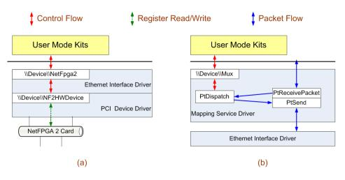
Figure 6: (a) Register Read/Write. (b) Packet Intercept/Inject.
