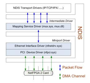
Figure 2: The structure of the kernel mode drivers.
