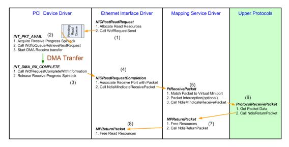
Figure 5: Packet receiving procedure.
