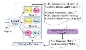
Fig. 1. Control loop for application placement (adapted from [6]).
