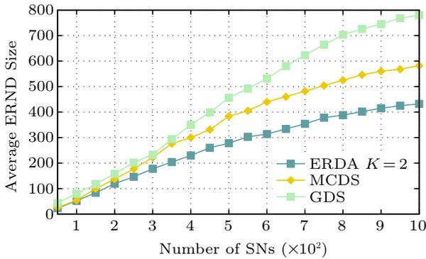
Fig.12. Average numbers of EHRs deployed compared with MCDS and GDS.
