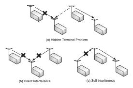
Fig. 2: Examples of collision types in wireless network.
