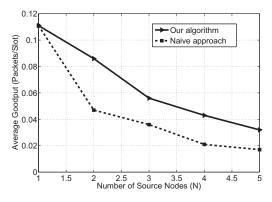
Fig. 10: Goodput comparison of scheduling algorithm and traditional broadcast mechanism in a fixed network.
