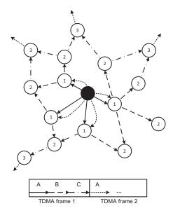
Fig. 3: Barrage relay network broadcast protocol for a three time slot TDMA frame format. The source node is black while relay nodes are numbered by their distance in hops from the source.
