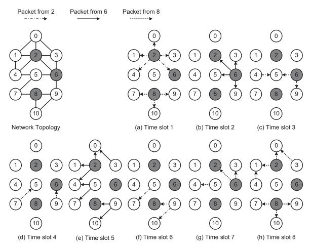
Fig. 7: Scheduling result about packets transmission in the first eight time slot with three source nodes(2, 6 and 8 in gray) in a barrage relay network. The transmission of packets from different source nodes are presented with different kinds of lines.
