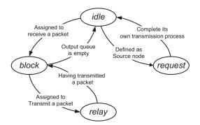
Fig. 6: Status transition in the process of scheduling.
