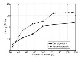
Fig. 8: Latency comparison of scheduling algorithm and the naive broadcast mechanism.
