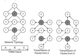
Fig. 5: Barrage relay process in a multi-source(node 2 and 8 in gray) broadcast scenario with naive approach.
