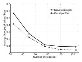
Fig. 9: Goodput comparison of scheduling algorithm and traditional broadcast mechanism with different size of network.
