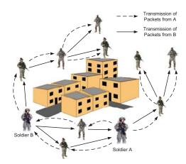
Fig. 1: A possible multi-source broadcast scenario in tactical field. Soldier A and B are broadcasting live-streaming videos captured by their camera.
