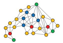
Fig. 4: Three unicast flows in a BRN. Source, destination, relay, and buffer nodes are colored green, red, blue, and yellow, respectively.
