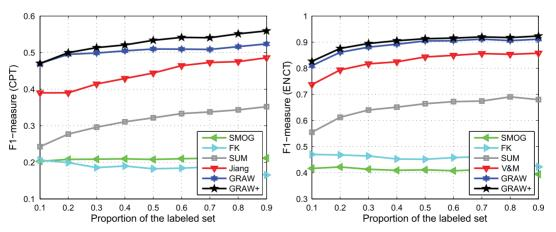
FIG. 5. The average F1-measures of the seven methods on both data sets (Jiang is running on CPT only, while V&M is running on ENCT only) with the labeling proportion varied from 0.1 to 0.9 step by 0.1. [Color figure can be viewed at wileyonlinelibrary.com]
